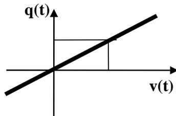
$$C = \frac{q(t)}{v(t)} = \frac{\Delta q}{\Delta v} = \frac{dq}{dv} = \text{Costante}$$
