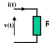
$$R_{\text{resistenza}} = \frac{\text{Tensione}}{\text{Corrente}}$$
